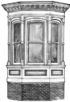
Figure 6: A polygonal bay window, typical of the Italianate and Second Empire Styles
