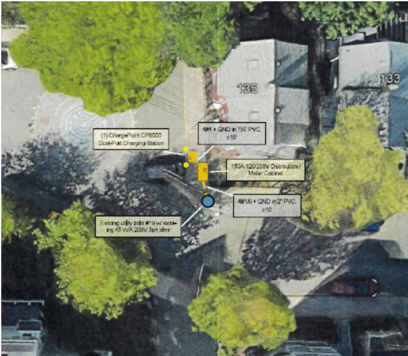
Closer view of the proposed equipment cluster at 135 Hudson Street. The corner area adjacent to Pole 202/19 functions as a pedestrian crossing point, particularly in winter when snowbanks restrict other crossing options. A cabinet position along the curb downstream of the charger pedestals would minimize sidewalk obstruction while preserving the corner crossing.
