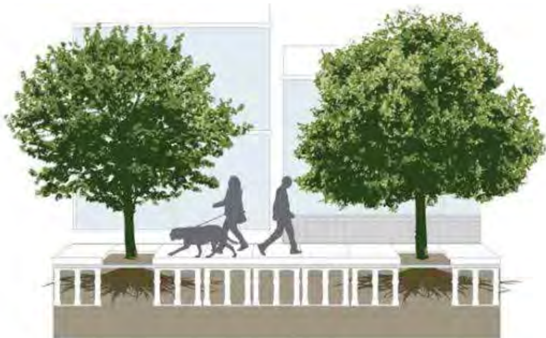
Figure 13.2.4 (b) Structural Cell Example
