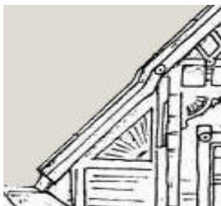
Figure 13: Trim work in gable.
