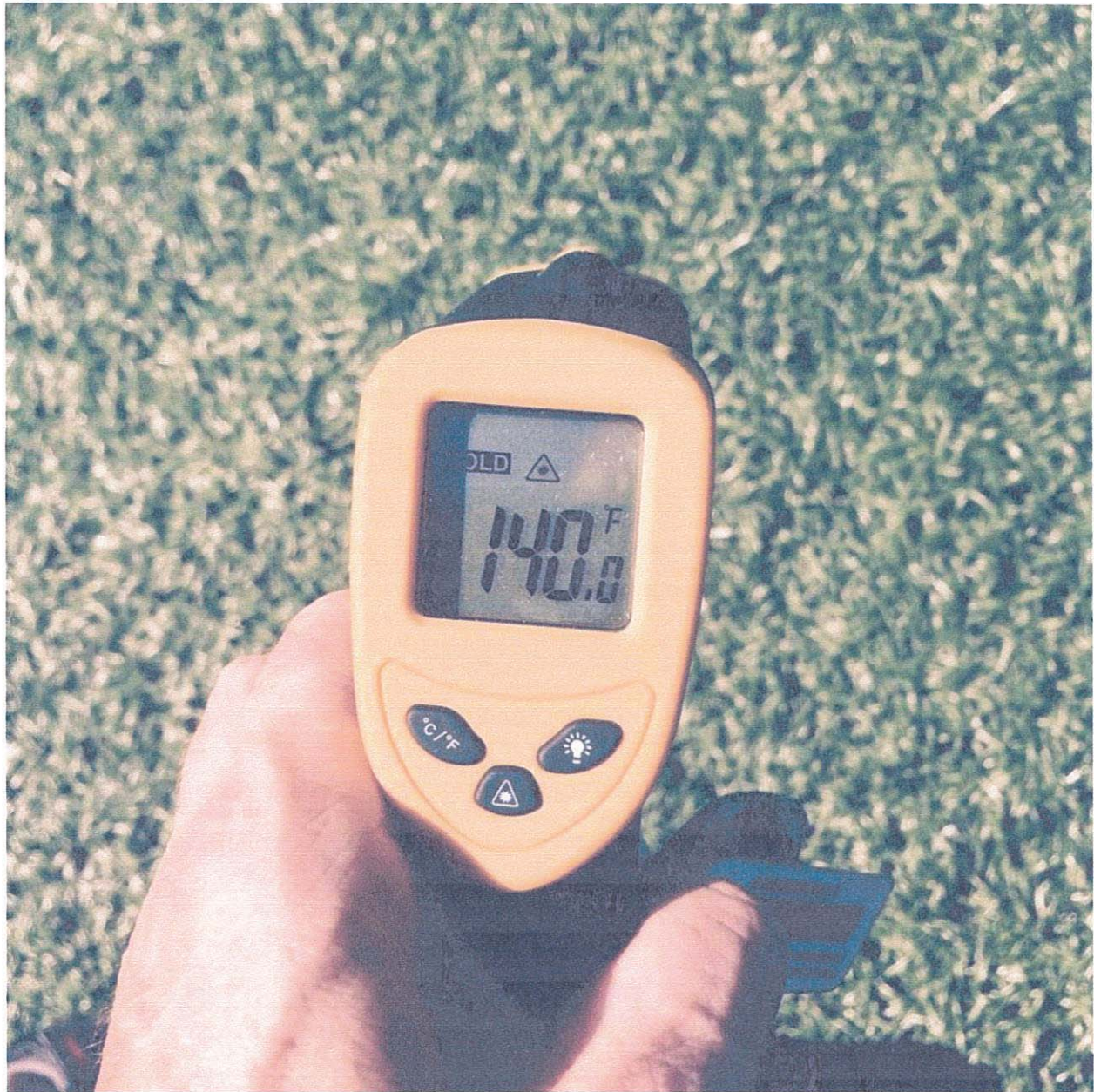
East Somerville Community School artificial turf field, Sept. 9, 2015, 2:30 p.m., 93 deg. air temp
