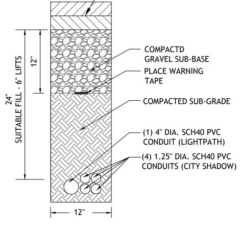
TRENCH/DUCT BANK DETAIL ON SIDEWALK
