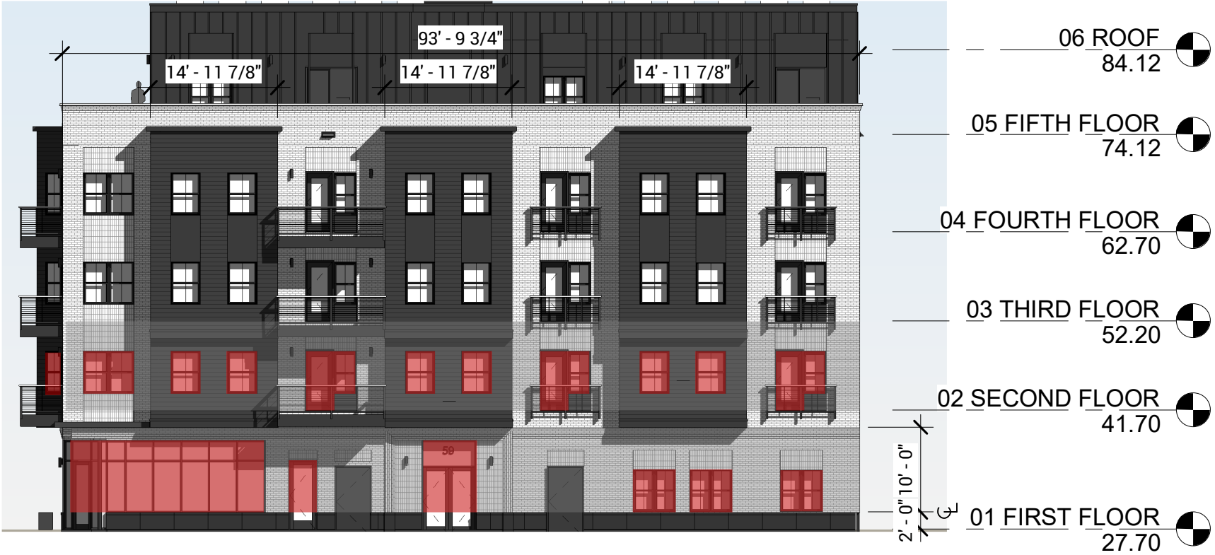
2 ELEVATION - BOW PLACE GLAZING 1/16" = 1'-0"
