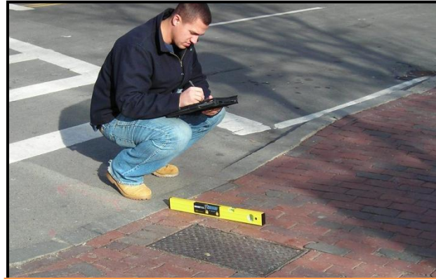
Recording ramp slope in field
