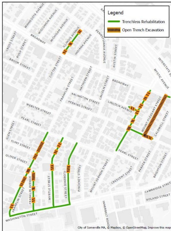
Figure 1. Sewer Pipeline and Manhole Rehabilitation
