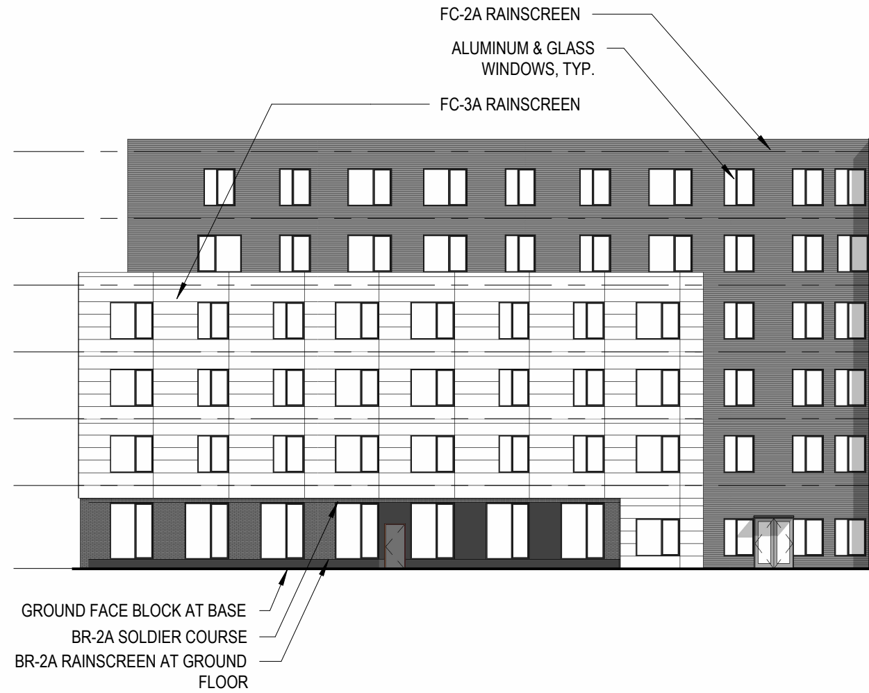
1 BUILDING A - ALCOVE NORTH ELEVATION 3/64" = 1'-0"
