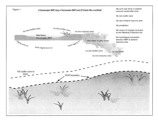
Alternatively, suppose the entire stormwater management system, including the water quality swale, infiltration basin, and riprap outlet, is constructed for stormwater management purposes in the Buffer Zone in accordance with the Stormwater Management Standards on or after January 2, 2008. As with the earlier example, no additional wetland resource area or Buffer Zone is created solely as a result of the installation of the stormwater management system. See Figure 2.
