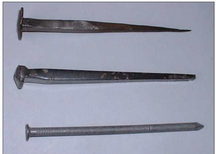
Figure 3 – Top: Handmade nail; Middle: Cut nail; Bottom: Wire nail
